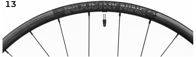
2020-Present | 1/1 Trail Carbon 28mm IW | 29" ERD 597 28H 29" DS 296mm | Non-DS 298mm
