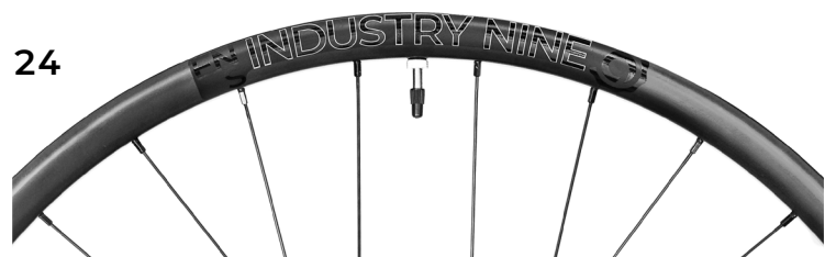
2020-Present | 1/1 Enduro S Carbon 31mm IW | 27.5" ERD 560 | 29" ERD 598 28H 27.5" DS 277mm | Non-DS 279mm 28H 29" DS 296mm | Non-DS 298mm
