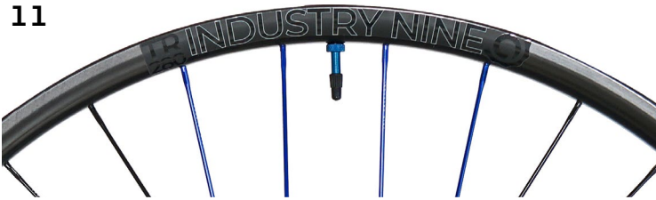
2020-Present | Trail 280 Carbon 28mm IW | 29" ERD 598 24H 29" DS 299mm | Non-DS 295mm 32H 29" DS 297mm | Non-DS 299mm
