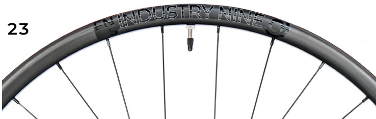
2020-Present | HYDRA Enduro S Carbon 31mm IW | 27.5" ERD 560 | 29" ERD 598 28H 27.5" DS 285mm | Non-DS 285mm 28H 29" DS 303mm | Non-DS 303mm
