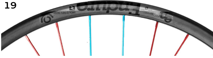
2015-16 | Enduro Carbon 26mm IW | 27.5" ERD 556 32H 27.5" DS 278mm | Non-DS 280mm
