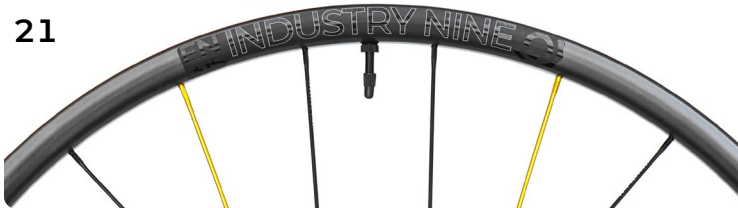
2020-Present | Enduro 315 Carbon 31.5mm IW | 27.5" ERD 562 | 29" ERD 599 24H 27.5" DS 278mm | Non-DS 280mm 32H 27.5" DS 280mm | Non-DS 282mm 32H 29" DS 299mm | Non-DS 300mm
