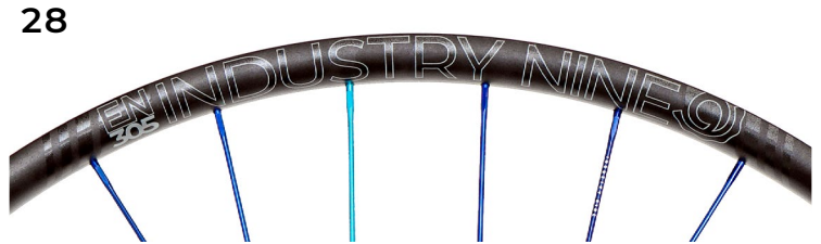
2021-Present | Enduro 305 V3 Alloy | Rim + Graphic Change 30.5mm IW | 26" ERD 539 | 27.5" ERD 565 | 29" ERD 603 32H 26" DS 268mm | Non-DS 270mm 32H 27.5" DS 280mm | Non-DS 282mm 32H 29" DS 300mm | Non-DS 302mm
