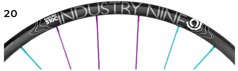
2017-19 | Enduro 310 Carbon | Rim + Graphic Change 30.5mm IW | 27.5" ERD 557 | 29" ERD 596 24H 27.5" DS 282mm | Non-DS 276mm 32H 27.5" DS 278mm | Non-DS 280mm 24H 29" DS 299mm | Non-DS 295mm 32H 29" DS 297mm | Non-DS 299mm
