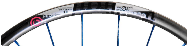
2013-14 | Trail Carbon 21.0mm IW | 27.5" ERD 549 | 29" ERD 586 24H 27.5" 274mm | Non-DS 270mm 32H 29" DS 291mm | Non-DS 293mm
