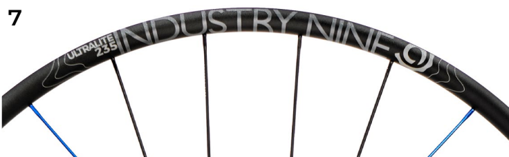
7 2017-19 | UltraLite 235 Alloy | Rim + Graphic Change 23.5mm IW | 27.5" ERD 563 | 29" ERD 602 24H 27.5" DS 281mm | Non-DS 277mm 24H 29" DS 300mm | Non-DS 296mm
