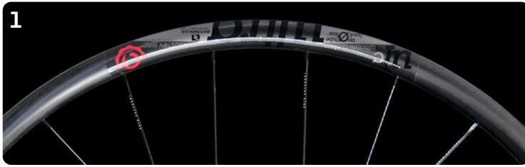
1 2013-14 | UltraLite Carbon 21.3mm IW | 29" ERD 592 24H 29" DS 296mm | Non-DS 293mm
