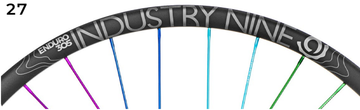
2017-19 | Enduro 305 V2 Alloy | Graphic Change 30.5mm IW | 26" ERD 532 | 27.5" ERD 560 | 29" ERD 597 32H 26" DS 266mm | Non-DS 268mm 32H 27.5" DS 278mm | Non-DS 280mm 32H 29" DS 297mm | Non-DS 299mm
