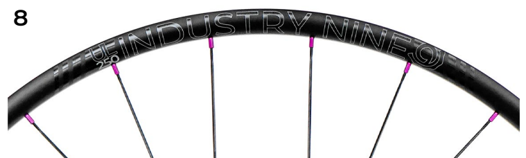
8 2020-Present | UltraLite 250 Alloy 25mm IW | 27.5" ERD 566 | 29" ERD 603 24H 27.5" DS 282mm | Non-DS 277mm 24H 29" DS 301mm | Non-DS 297mm
