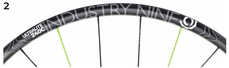
2 2015-19 | UltraLite 240 Carbon | Rim + Graphic Change 23.5mm IW | 29" ERD 599 24H 29" DS 299mm | Non-DS 295mm
