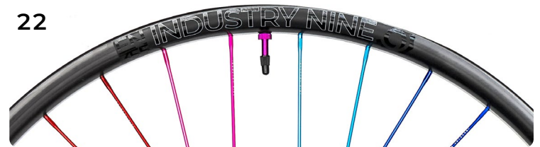
2020-Present | Enduro 355 Carbon 31.5mm IW | 27.5" ERD 561 | 29" ERD 599 32H 27.5" DS 280mm | Non-DS 282mm 24H 29" DS 299mm | Non-DS 295mm 32H 29" DS 299mm | Non-DS 300mm
