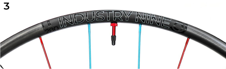
3 2020-Present | UltraLite 280 Carbon 28mm IW | 29" ERD 602 29" DS 300mm | Non-DS 296mm
