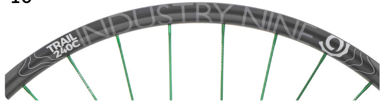
2015-19 | Trail 240 Carbon | Rim + Graphic Change 27.5" 23.5mm IW ERD 556 | 29" 26mm IW ERD 599 24H 27.5" 280mm | Non-DS 276mm 32H 29" DS 297mm | Non-DS 299mm
