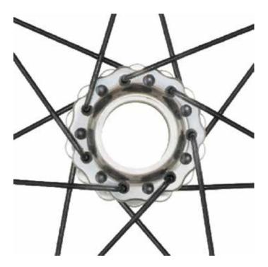
Follow spoke placement in the hub flange orientation as pictured. Note the "ridge" and the "valley" of the scalloped flange shaping.
