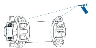
**Front Endcap Installation** - Coat the seal of the bearing and the o-rings inside the endcaps with grease before pressing the endcaps into the hub.
