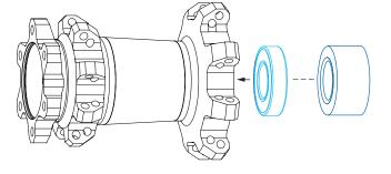
**Rear Hub Assembly** - Start by pressing the drive side bearing into the drive side of the hub using a bearing press.
