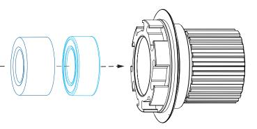
BEARING LAYOUT CHART HUBSHELL DRIVE SIDE NON-DRIVE SIDE 6 Bolt Mountain Front 1 x 61804 1 x 61804 6 Bolt Mountain Rear 1 x 15307 1 x 61804 Center Lock Mountain Front 1 x 18307 1 x 18307 Center Lock Mountain Rear 1 x 15307 1 x 61903 Lefty Front Mountain 1 x 61805 1 x 61902 FRFFHUB INBOARD OUTBOARD Hydra XD + HG 1 x 152610 1 x 15267 Micro Spline 1 x 152610 2 x 6802
