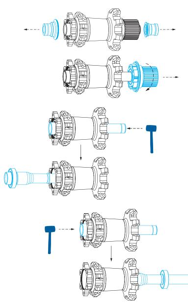
**Rear Hub Disassembly** - To disassemble your torch hubs you need to first remove the endcaps from the axle. The endcaps are held in place with a rubber o-ring seated in the endcap. endcaps do not require tools for removal.\*
