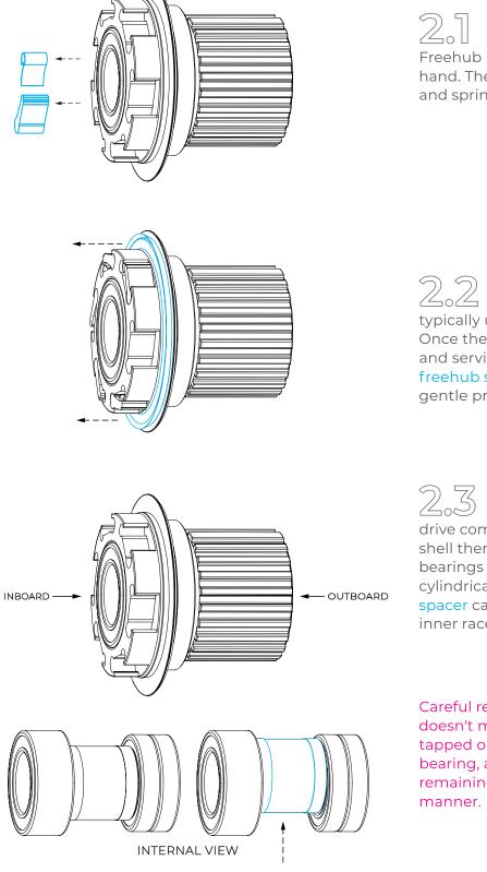
**Freehub Disassembly + Service -**Freehub body components are easily removed by hand. The pawls and springs slide out of the pawl and spring pockets.
