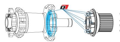
**Freehub Installation on Hubshell** Apply a few drops of Dumonde Tech freehub grease to the drivering and pawls. Apply a drop of oil to the freehub seal.
