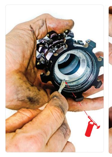
12 Apply a layer of grease on the drive ring. gently place the freehub assembly into the hubshell to get it straight before pushing any further. ratchet the mechanism to ensure it's lined up and not crooked in the bore. If you press it in while it's crooked, you may damage the pawl springs. Try to free wheel the freehub as you are pressing it in as that will reduce the likelihood of damaging the springs. If it feels rough, you may need to push the freehub out and start again.
