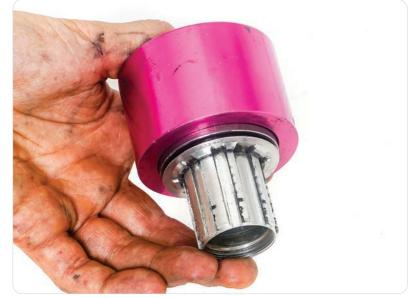
**8** Use a bushing or section of pvc to press the 61808 bearing back on. Reinstall the bearing retainer circlip.
