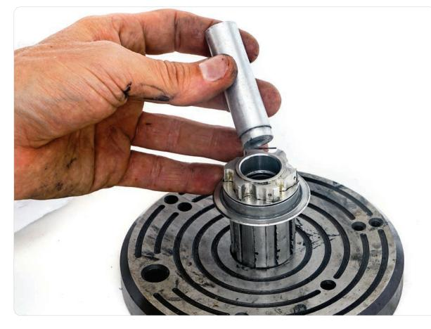
**6** To remove the two inner bearings, use a punch or dowel to catch the inner races.
