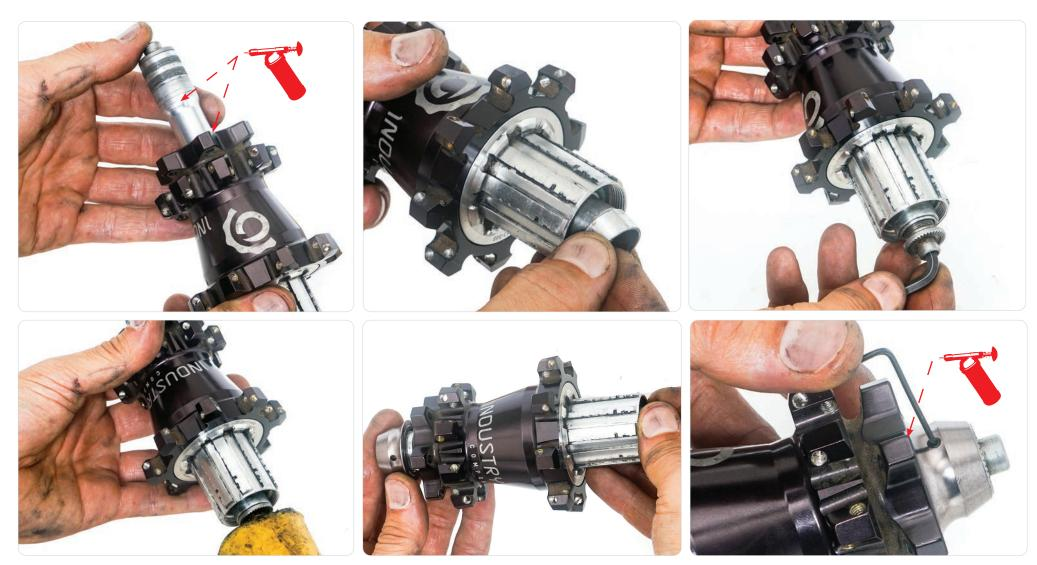
**14** Apply grease to inner bearing races as well as the bearing seats on the axle. Apply grease to the threads for the adjustable dustcover. Reapply blue loctite to the 1.5mm grub screw. Install the axle and install drive side endcap. Install adjustable dustcover until there is a small amount of lateral play.
