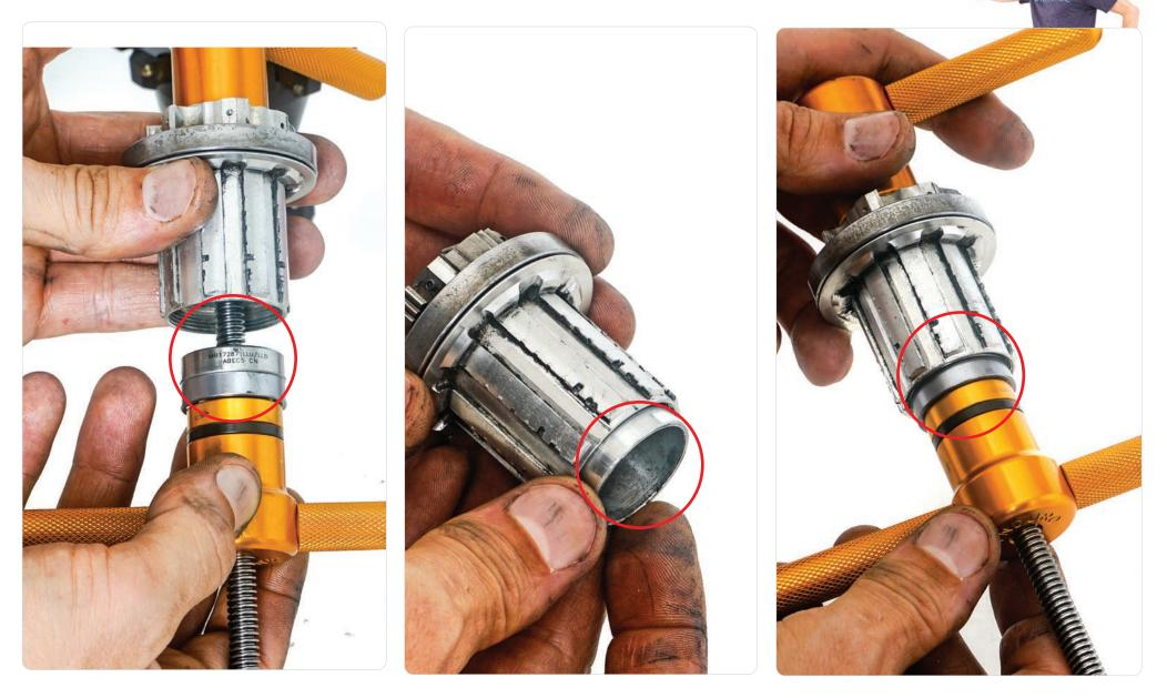
II Use a bushing to press the first bearing all the way into the freehub.Apply a light film of grease to the bearing spacer and push it in.Install the second bearing.
