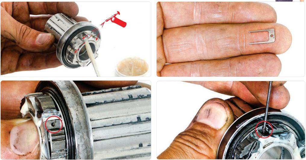
**9** Put a small dab of fresh grease in all six of the pawl pockets before placing each pawl back in.
