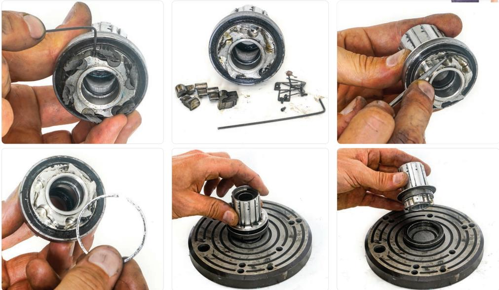
**5** Wipe any excess grease from around the pawls. Use a .050" allen to loosen the six allen bolts that hold the pawl springs in place. Wipe down the pawls and pawl pockets.
