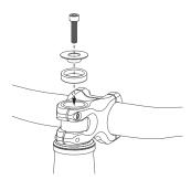
Install top cap according to the fork manufacturer's specifications.
