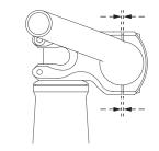
Ensure the gap is even on top and bottom between the faceplate and stem body.
