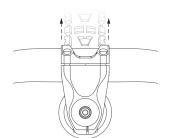
Ensure stem and bars are aligned with the front wheel.
