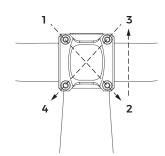
Tighten bolts to 5-6 Nm. Do not exceed handlebar manufacturer's specified torque.
